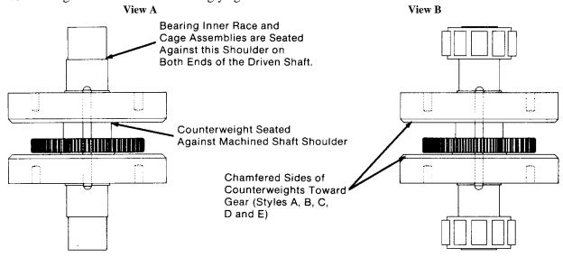
Figure 4.8 Installation of second counterweight and bearing inner races with roller cages on driven shaft.
