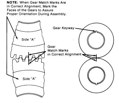
Figure 4.10 Match mark alignment of properly assembled gears.
