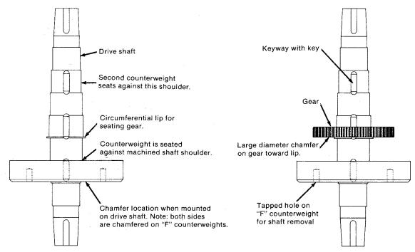
Figure 4.4 Mechanism shaft (key features)
