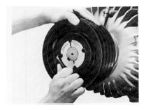
Tighten screws alternately
