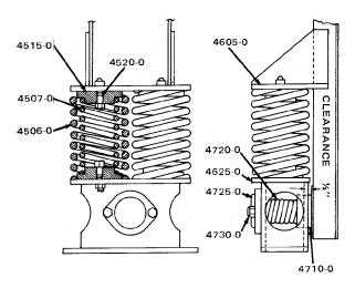
Figure 2.1 Fixed bracket mounting with inner and outer steel coil springs.
