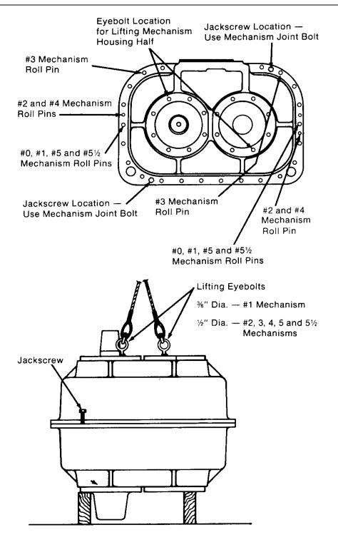
Figure 4.2 Method of dismantling housing halves (lower) Roll pin, eyebolt and jackscrew locations (upper)
