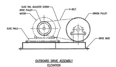
Figure 2.2 Drive motor mounted independently.
