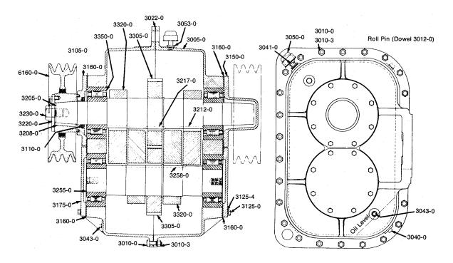
Figure 4.1 Typical Cross Section through Low-Head Mechanism.
