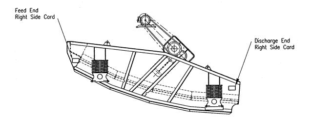
Locate Throw Cards in the same position on both Feed End corners and both Discharge End corners.
