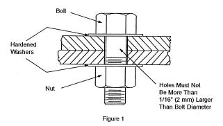
Figure 1: Cross section showing layout of bolts, washers and nuts
