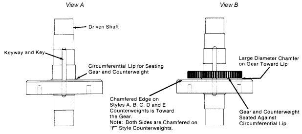
Figure 4.7 Installation of second counterweight and gear on driven shaft.
