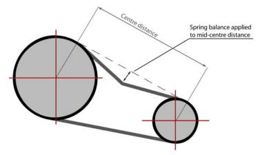
Figure 3: Belt tensioning diagram
