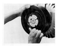
Removing a Taper Lock® bush
