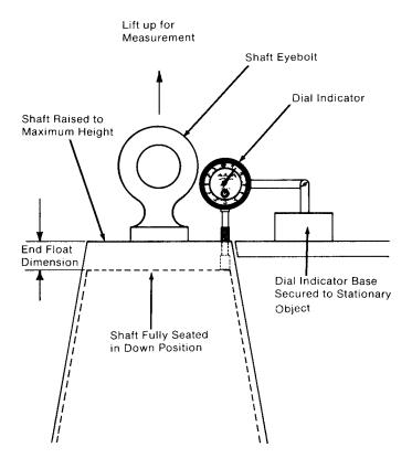
Figure 4.11 Dial indicator arrangement for checking shaft end float.
