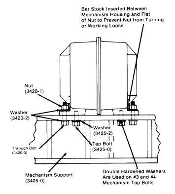
Figure 4.12 Mechanism mounting, No.2, No.3 and No.4.
