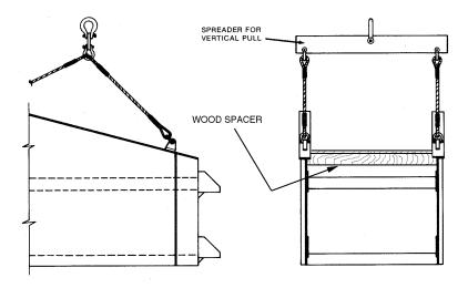
Figure 1.1 Use of spacers and spreaders when lifting the screen
