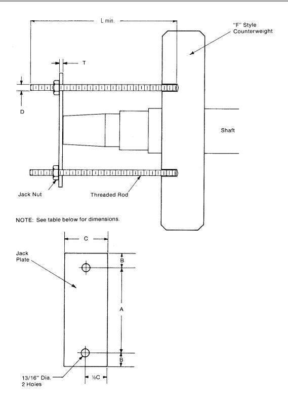
Figure 4.3 Method of pulling 'F' type counterweight off shaft.
